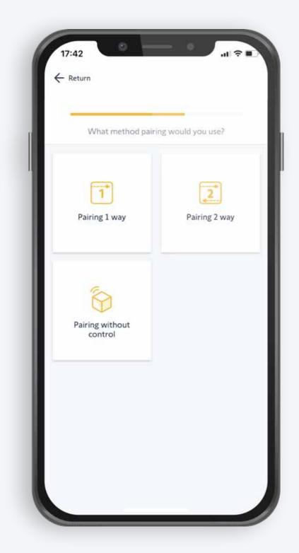
10. Tap the desired pairing mode; indicate if the motor is programmed with a 1-way or a 2-way transmitter, or if it is still in factory mode
